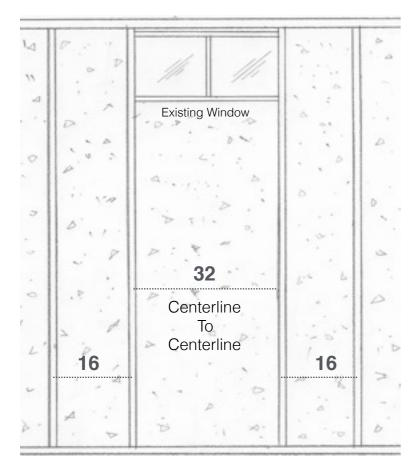
The Chase Window requires a 32" on center stud spacing in the area that the window is to be installed. Be as accurate as possible on the 32 inch spacing as this will affect the window fit. The opening between the two studs surrounding the window should be approximately 30.5".
