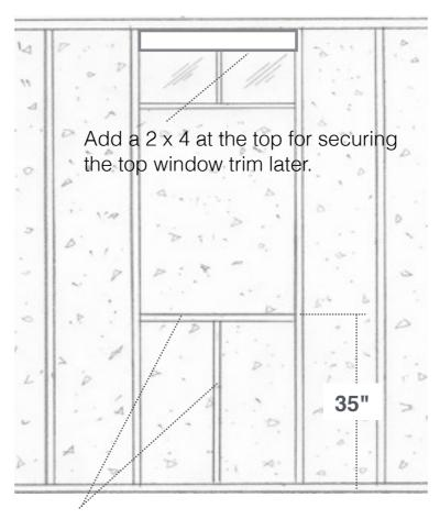
Using a level install a 2 X 4 sill and support 35" above the floor.
